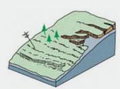
Extremely slow movement of surficial soil layers on a soil (typically less than 1 m deep). Over time, material loosened by creep can become source material for shallow slides and debris avalanche.
