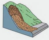
Occurs when a slope failure consists of an unsorted mix of rock and soil, regardless of moisture (Schuster & Crandell, 1984). With the addition of water in a channel, can become debris flows.
