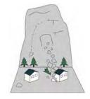
Rapid movement of shattered and pulverized fragments of bedrock. Travels much faster and further than rock fall. Can block rivers and create landslide-generated waves.
