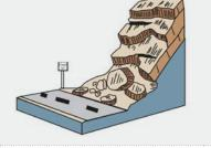
Rolling, sliding, and stopping of rock fragments falling off slopes. Occurs in mountainous regions and can form talus slopes due to repeated events. Can become rock avalanches as they erode.
