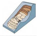
Rock (and debris/earth) slides involve the movement of rock/debris/earth that largely remain on the sliding surface. Sliding (failure) surfaces can be planar (translational) or curved (rotational), and are often a combination.
